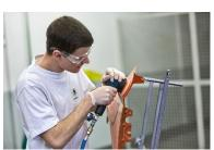
New Student Concept Car named the ŠKODA MOUNTIAQ Finishing touches for the ŠKODA MOUNTIAQ: an apprentice is using a buffer to polish the Orange Sunset paint finish to a fine sheen.
