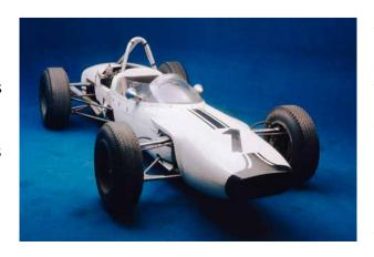
A formula racing car was built in Vrchlabí in the 60s as well. The ŠKODA F3 prototype was powered by a modified ŠKODA 1000 MB engine. Its 1.0-litre four-cylinder with an aluminium block generated a power output of up to 66 kW, allowing the car weighing just 410 kg to reach 210 km/h.
