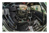
The safety devices of the ŠKODA FABIA Rally2 evo Safe and functional: The cockpit of the ŠKODA FABIA Rally2 evo with its roll cage and racing seats with head wrap around
