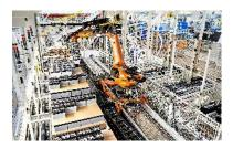
Robot delivers just-in-sequence parts directly to the production line at the ŠKODA AUTO plant in Kvasiny In Kvasiny, starter batteries are placed on pallets near the assembly line where they are ready for use when required. This is in contrast to conventional sequencing, which instead sees the batteries being fetched from the parts warehouse when they need to be fitted into the cars.
